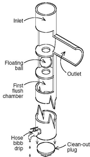
**Fig. 7: First-flush diverter (Texas Water Development Board 2005)**
