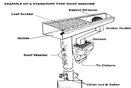
*Fig. 5: Roof washer (Van Giesen and Carpenter 2009)*
