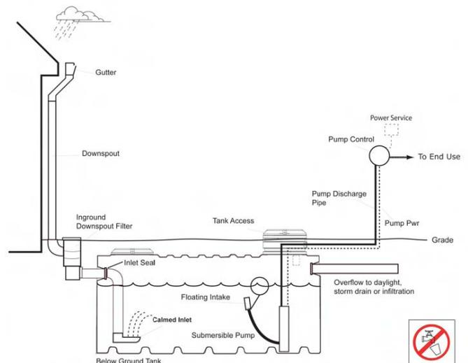
Fig. 3: Below ground system (Van Giesen and Carpenter 2009)
