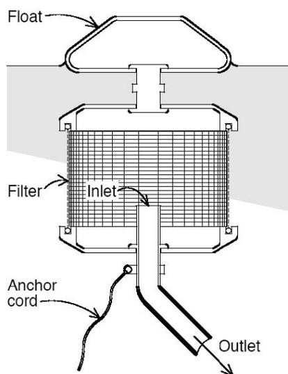
**Fig. 9 Floating intake filter (Texas Water Development Board 2005)**
